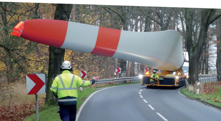
The Bladelifter can even transport rotor blades round tight bends
